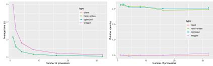
Shared memory machine (256 Gb), two Intel Xeon E5-2683 v4 (16 cores at 2.10 GHz). Ran 30 times with the following software: CentOS 7, Python 3.6.3, mpi4py 3.0.2, OpenMPI 2.6.4.
